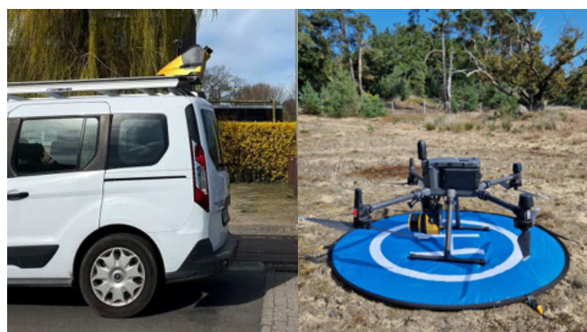
YellowScan Surveyor Ultra integrated for mobile and airborne mapping
