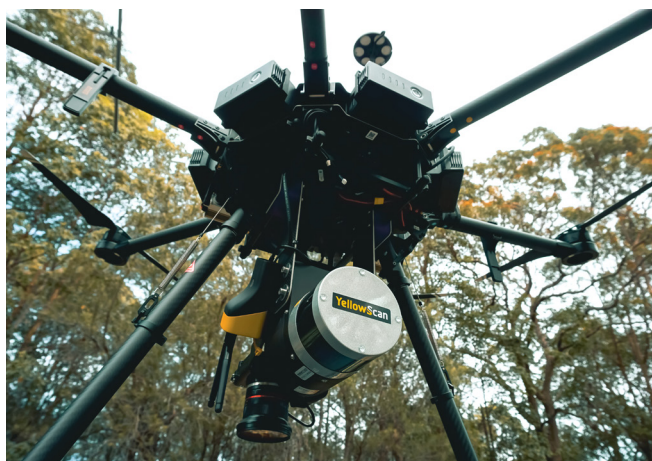
YellowScan Surveyor, LiveStation and RGB camera on a M600 from DJI
